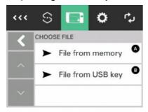
Selecting the A or B area because you can print an object taken from the internal memory of the machine (A) or from the connected USB key (B).
