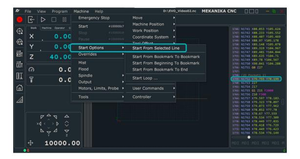
At the bottom of this section, you can find a **command line**, also called **MDI**, that is used to **type G-code manually and send it directly to the machine**. For instance, the command shown below will move the machine at maximal speed to the **working coordinates X50 and Y100**. If you want to know more about this, you can find all the information you need inside the PlanetCNC G-code documentation, which can be downloaded on the support page of our website.
