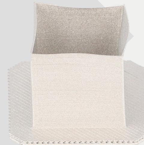
Figure 18: 0.4mm Wall Failure
