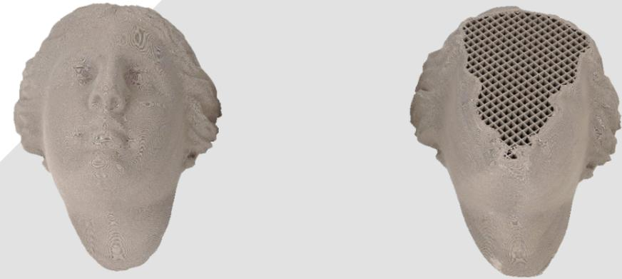
Figure 21: Mass Reduction Using Infill
