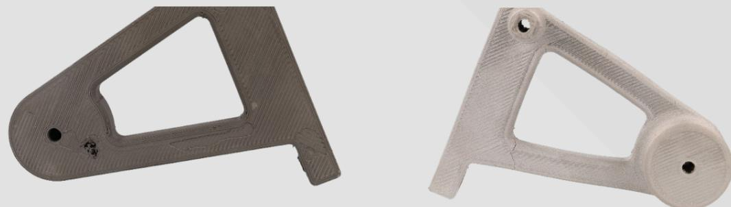
Figure 16: Damaged Bottom Surface and Resulting Top Cracks
