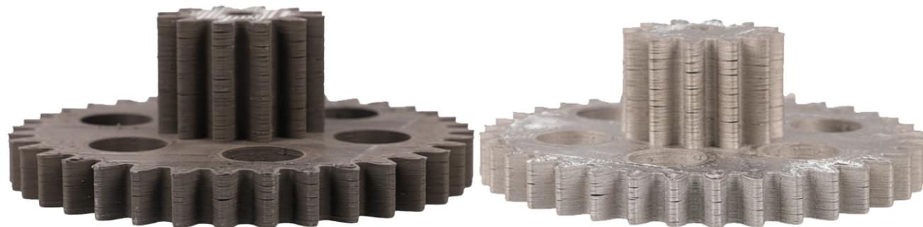
Figure 6: Print Delamination Become Sintered Cracks
