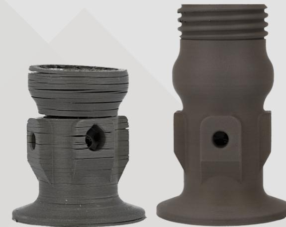
Figure 22: Cooling & Delamination Example
