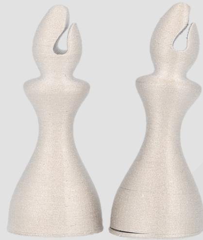
Figure 14: Warped Bottom Can Lead to Failure
